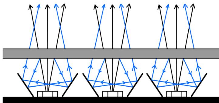
*General schematic of LED chips with integral reflector demonstrating linearity of beam.*
